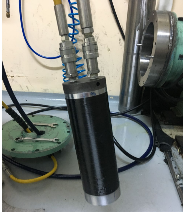
Figure 5. Hydrostatic Burst Pressure Setup
