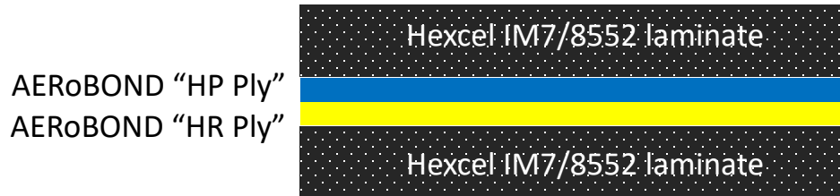
Figure 8. Configuration of AERoBOND laminates for mechanical testing.
