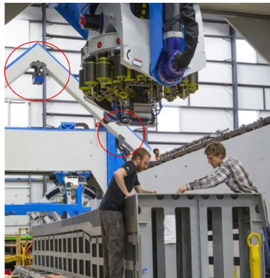
Figure 4. Automatic inspection of Boeing 777X component. Two guidance/inspection units circled in red.
