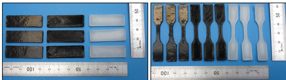
Figure 1: Flexural as well as DMTA test specimens - (a) Compression moulded composite; (b) 3D printed composite; (c) 3D printed LLDPE and Tensile test specimens - (a) Compression moulded composite; (b) 3D printed composite; (c) 3D printed LLDPE
