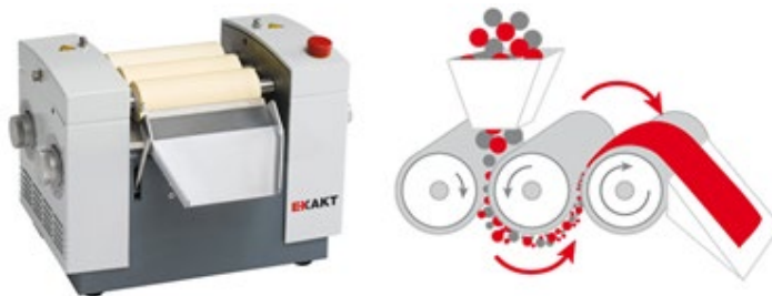
Figure 1: Three roll mill and illustration of dispersion using calendaring approach (Courtesy: www.exaktusa.com )
