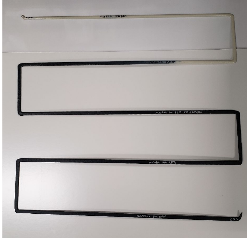
Figure 3. A 100 RPM sample printed with BAAM-B's dual-hopper.
