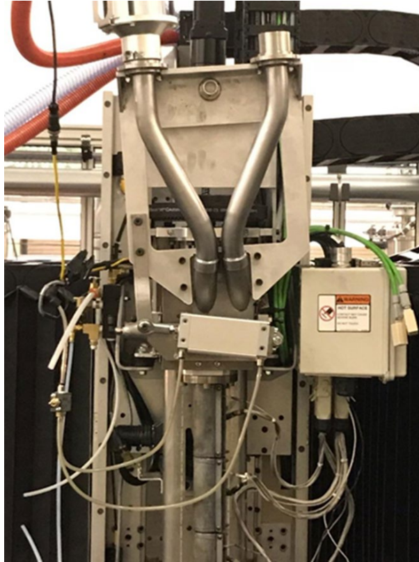
Figure 1. Image of the dual-hopper attachment and feeding tubes for BAAM-B.
