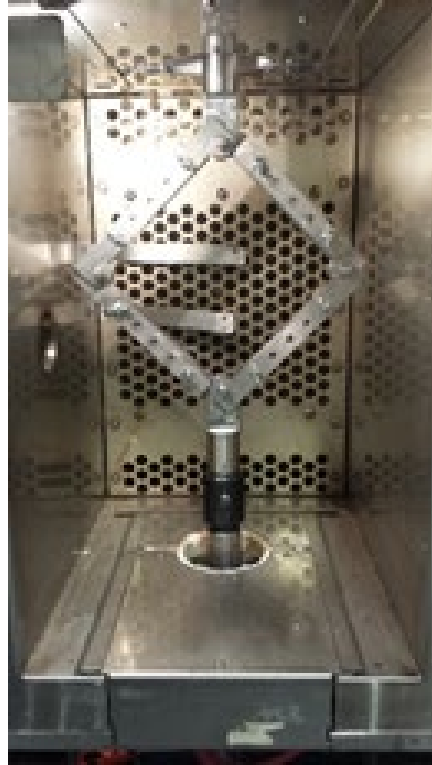
Figure 4. Temperature chamber used to characterize the prepreg material at forming temperature.
