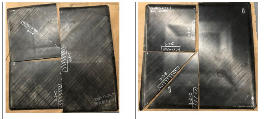
Figure 14- Section cut locations for geometry 2 (left) and geometry 3 (right)
