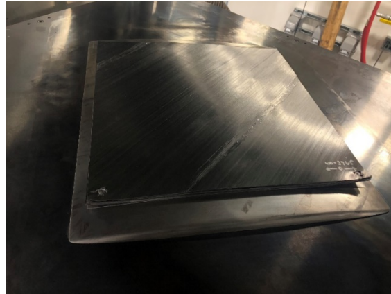
Figure 5 - Ply kit on the consolidation tool prior to fabrication
