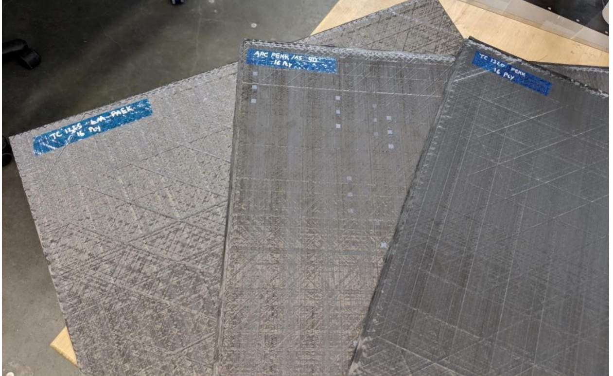
Figure 15. Quilting patterns emerge as more plies are laid down. The effect is exaggerated to unacceptable levels at high speeds.
