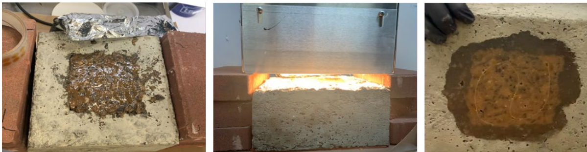
Figure 3. 4" x 4" x 4" prototype patch containing the ODiSI thermal sensing fiber, cured with the IR Heater. Image at right shows the bottom of the patch 1 hour after cure
