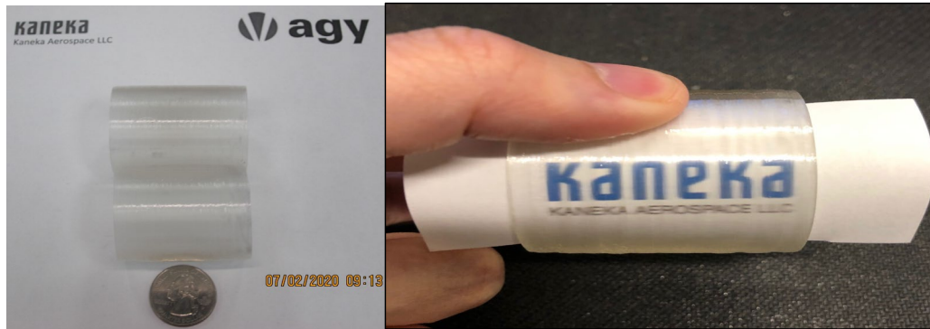
Figure 3. Demonstration articles filament wound on an aluminum alloy mandrel. Tube dimensions OD = 35 mm, wall thickness = 1.6 mm.
