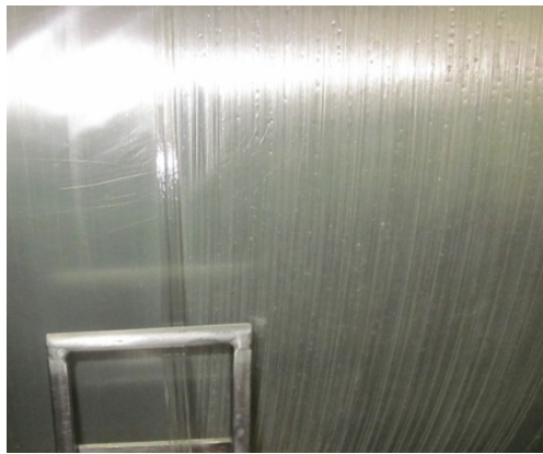
Figure 2. Filament winding of S-2 Glass roving and Kaneka 19-04-12 followed by cure and consolidation gives the clear UD composite (right).
