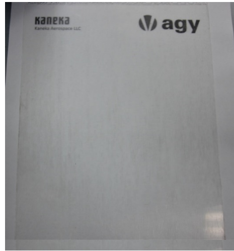
Figure 2. Filament winding of S-2 Glass roving and Kaneka 19-04-12 followed by cure and consolidation gives the clear UD composite (right).
