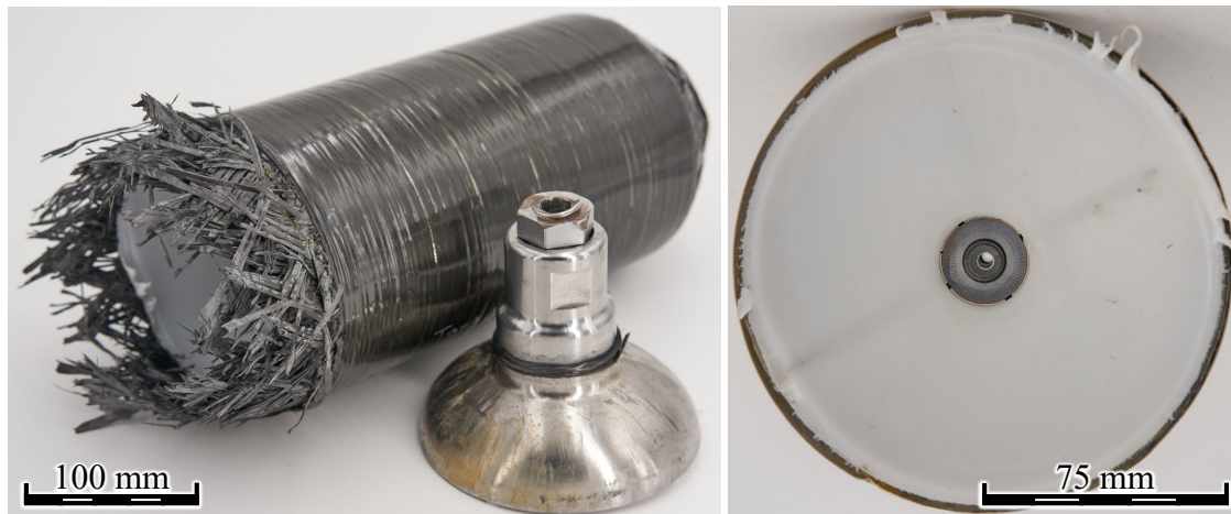
Figure 9. Damaged CPV after burst testing (left) and sheared liner (right).
