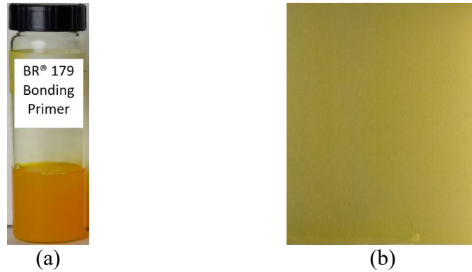
Figure 1. (a) BR ® 179 primer appearance; (b) Sprayed and cured BR ® 179 primer film at 5.1 μm (0.2 mil) thickness using Al 2024T3 Bare(FPL + PAA).
