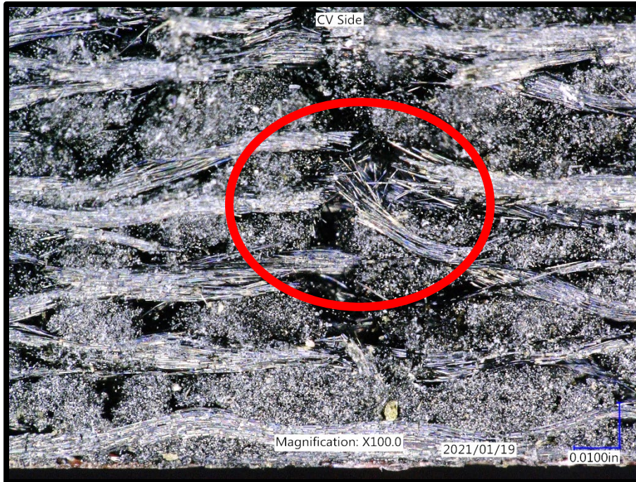
Figure 6 – Optical Image of Broken Fibers in Needle-Punched Laminate
