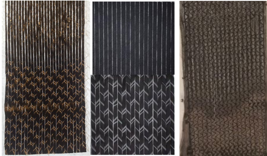
Figure 9. Left: Small-scale A&P prepreg without an attached veil. Middle: Small-scale A&P prepreg with an attached veil. Right: Small-scale VectorPly C-LA 1812 prepreg
