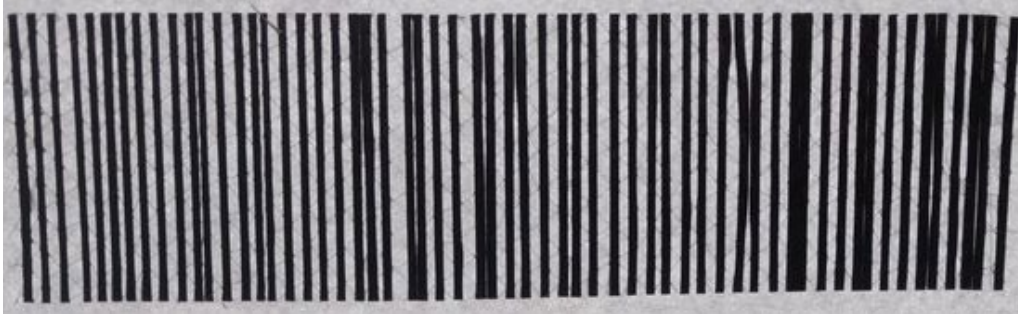
Figure 2. Severe tow separation and deterioration of structural integrity from the solvent-dip prepregging process.
