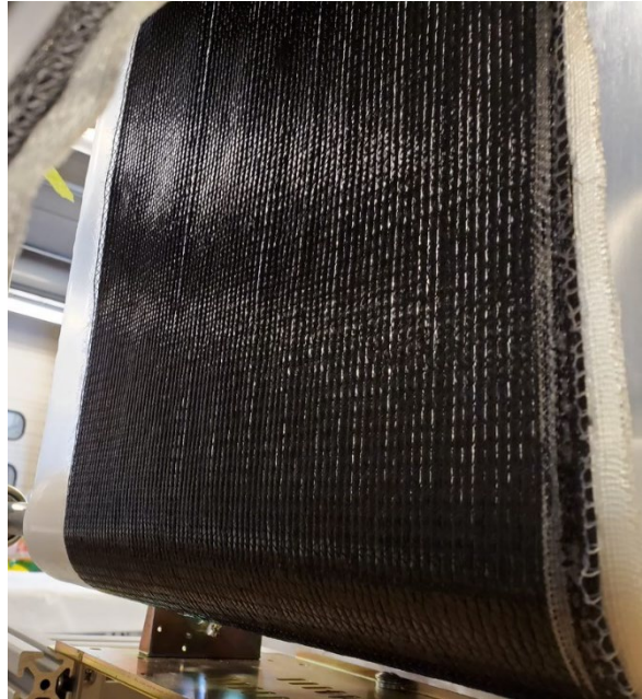
Figure 11: WWU UD prepreg after exiting the oven system.
