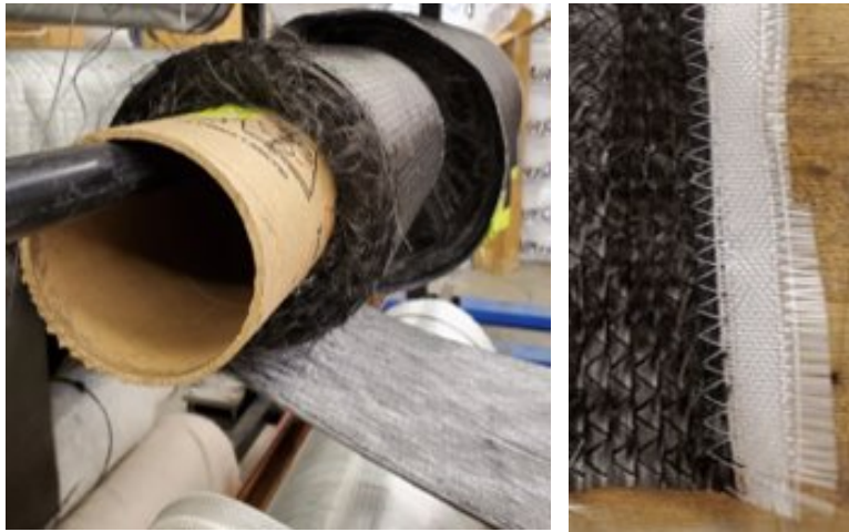
Figure 4: Left: Fiber fraying seen from damage tows after cutting. Right: Zig-zag pattern securing damaged tows to fiberglass tape.
