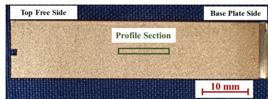
Figure 6. Profile measurement location for thin fin structure surfaces [8].
