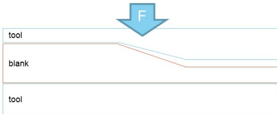
Figure 11: The top tool is first in contact with the thick part of the blank due to bulk factor
