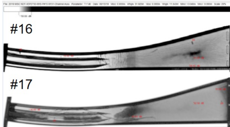
Figure 10: Comparative C-scan analysis between parts #16 and #17, highlighting the positive effect of asymmetrical IR preheat done on part #17
