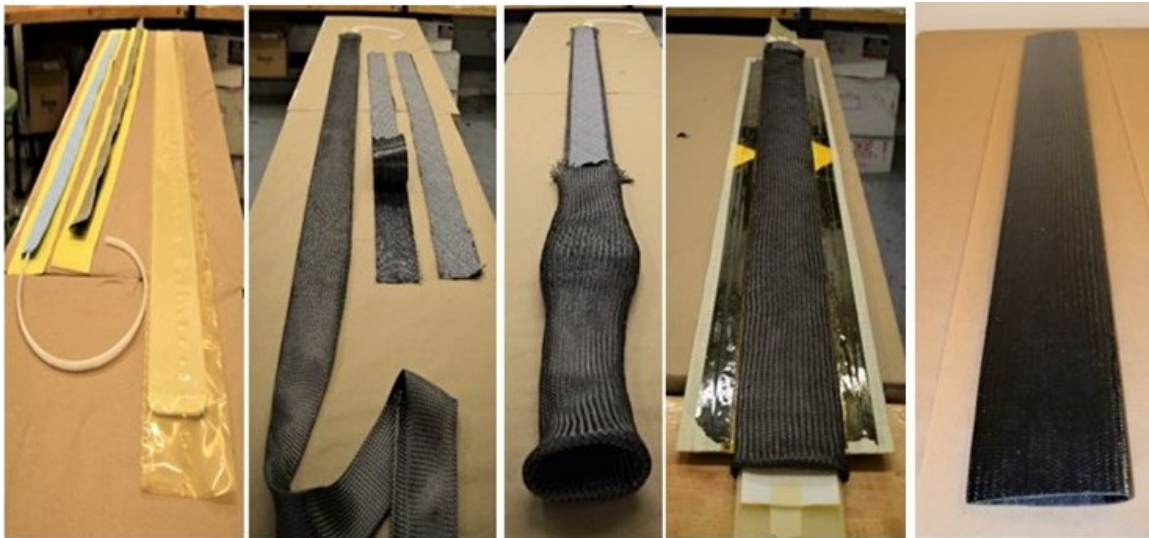
Figure 5. Adaptation of 1.6m manufacturing process to braided carbon fiber. From left to right shows the consumables, preform set-up, placement of the final ply, preform in mold, and the 1.6m carbon fiber airfoil.
