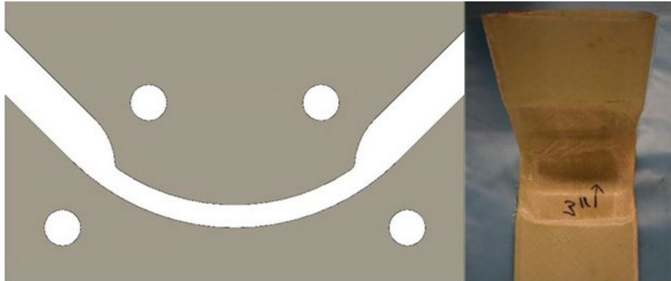
Figure 10. Trial 90 degree matched die set and resulting bend
