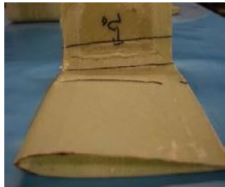
Figure 9. Buckling in preliminary trial 90 degree free bend of airfoil geometry
