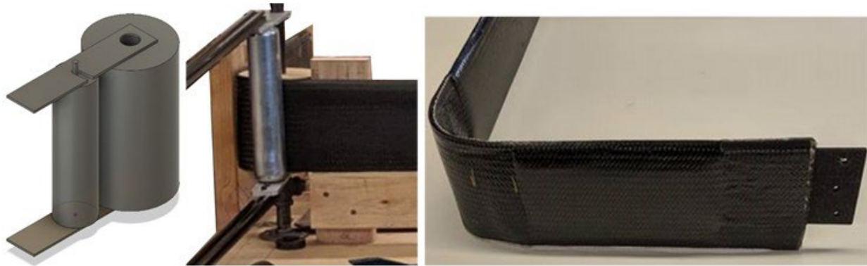
Figure12. Wiping die set and resulting double bend test article
